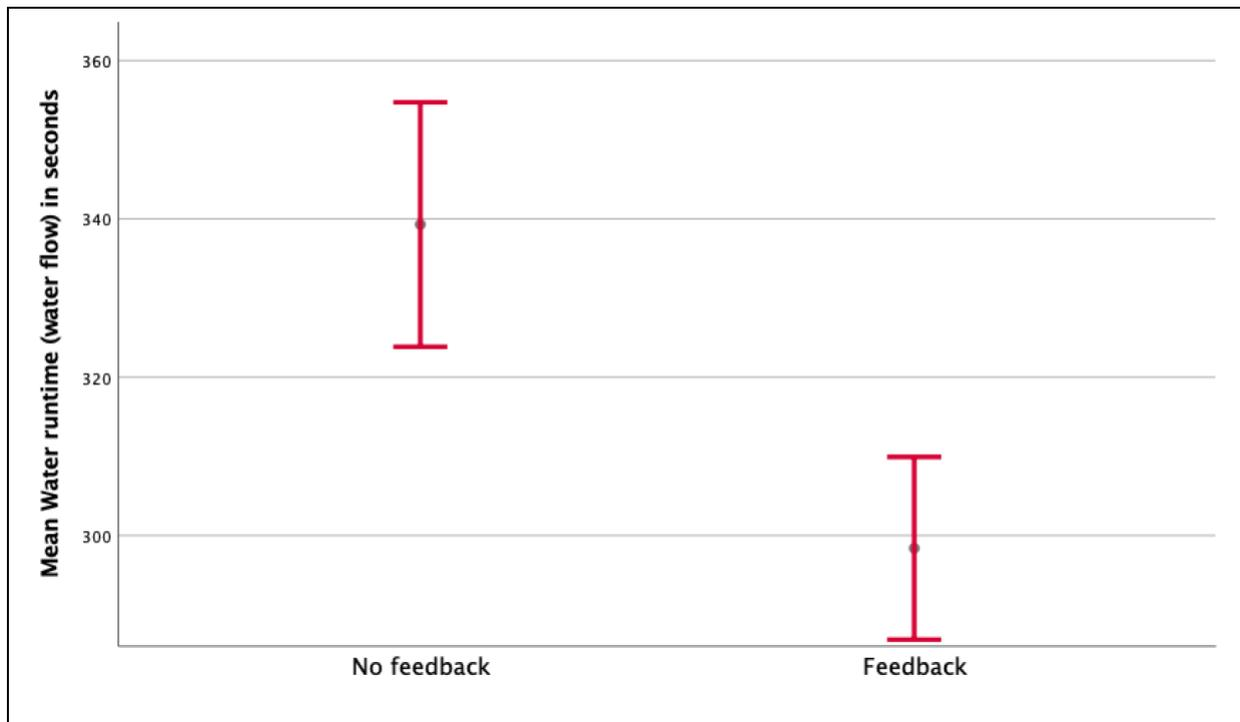
Fig.6. Error bar chart showing distribution of water runtime per shower at 95% CI in the control (no feedback) and treatment (feedback) groups (N=1,962).
