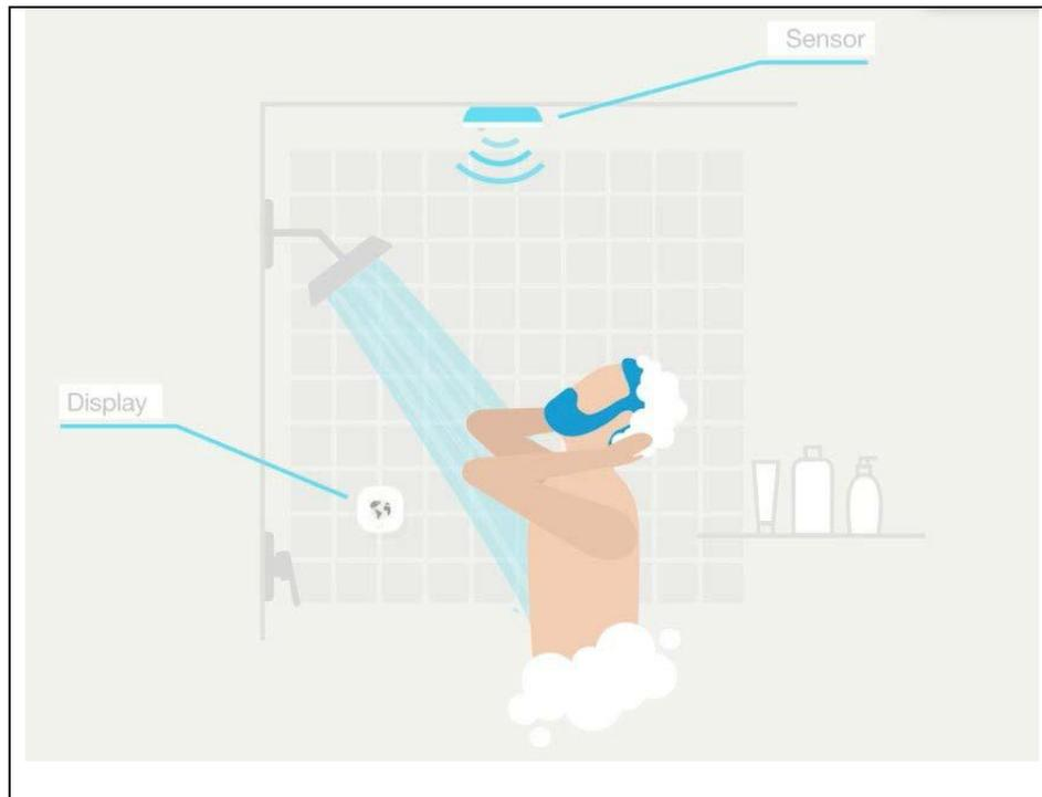
Fig.3. Location of the Display and the Sensor in the shower cabin. *Source: Aguardio ApS*
